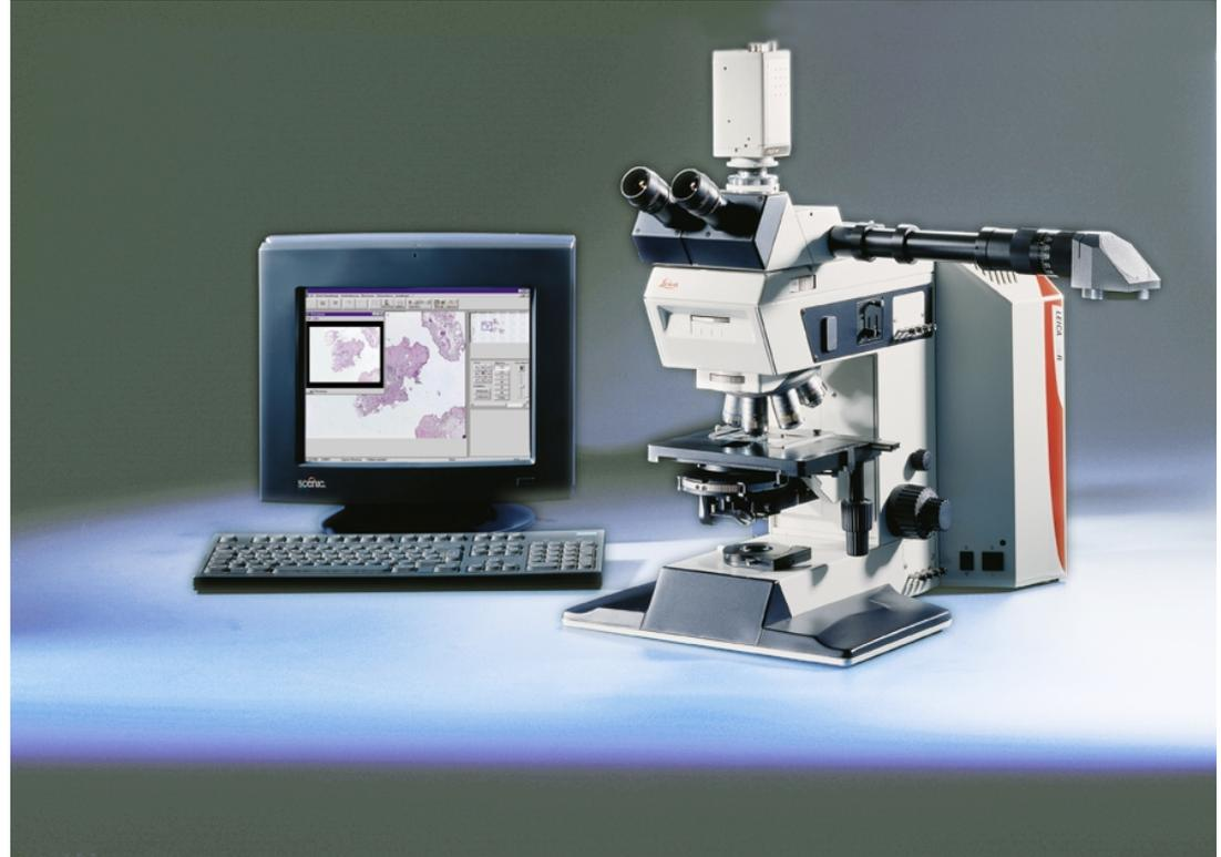
Fig. 1: Leica TPS 1 with remote controllable Leica DM RXA microscope, 3CCD camera, autofocus; server PC with specific hard- and software for image and data communication
